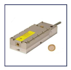
For generating high peak power ultraviolet pulses of a few hundred picoseconds, microchip lasers are economical, compact, and reliable. Microjoule UV pulses are generated from the harmonic conversion of the emissions from a passively Q-switched Nd:YAG microchip engine. The SNV and SNU series are designed for high average power, delivering multi-kW peak power at repetition rates up to 20kHz.
